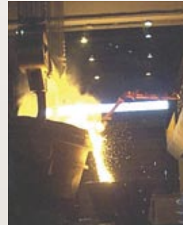
A high-tech tool at Republic's Lorain facility rakes slag from ladles of molten steel. The process lowers hydrogen levels in the melt and improves the quality of the steel's casting.
